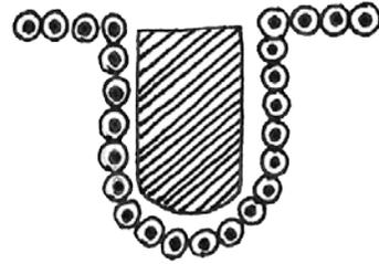
2) Lay out the first layer of tires where you want your walls. Build the south facing wall with glass.
